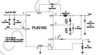
Work Mode 1: CS to GND with sensing resistor Fig. 1 Schematic
