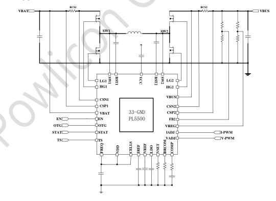
Fig. 1 Application Schematic
