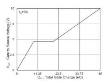
**Fig.4 Gate-Charge Characteristics**
