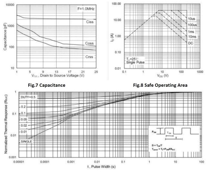
Fig.9 Normalized Maximum Transient Thermal Impedance
