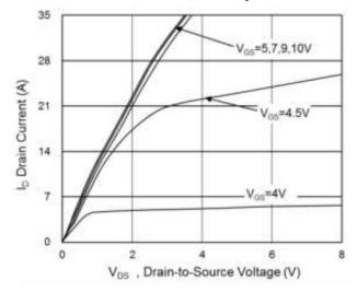
**Fig.1 Typical Output Characteristics**
