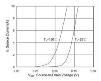
Fig.3 Forward Characteristics of Reverse Diode
