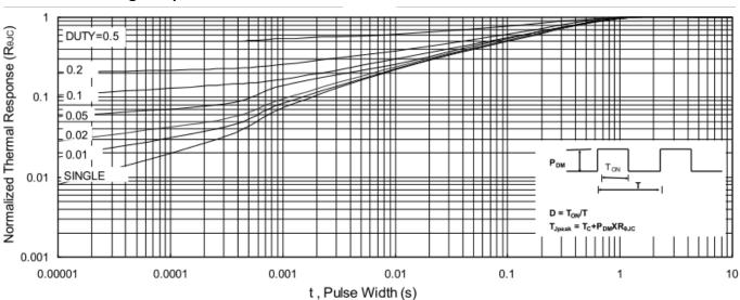
Fig.9 Normalized Maximum Transient Thermal Impedance
