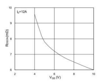
Fig.2 On-Resistance vs. G-S Voltage
