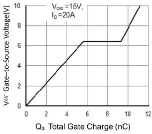
Fig.4 Gate-Charge Characteristics
