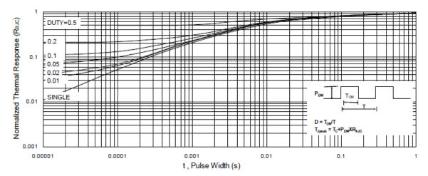
Fig.9 Normalized Maximum Transient Thermal Impedance
