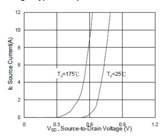
Fig.3 Forward Characteristics of Reverse Diode
