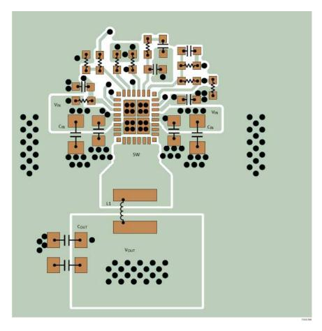
Figure 9. Example of Top Layer PCB Design
