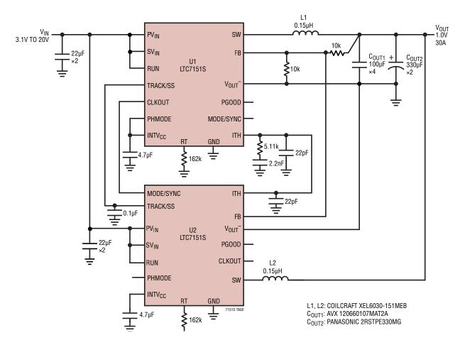
High Efficiency, Dual Phase 1.0V/30A Step-Down Supply
