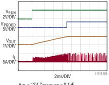
$\begin{array}{l} {\sf V}_{IN} \ = \ 12 {\sf V}, {\sf C}_{TRACK/SS} = 0.1 \mu {\sf F} \\ {\sf R}_{OUT} \ = \ 60 \Omega, \ {\sf L} \ = \ 0.15 \mu {\sf H}, \ f \ _{SW} \ = \ 1 {\sf M} {\sf Hz} \\ {\sf R}_{FB1} \ = \ 10 {\sf k} \Omega, \ {\sf R}_{FB2} \ = \ 10 {\sf k} \Omega \\ {\sf C}_{OUT} \ = \ 10 0 \mu {\sf F} \ + \ 2 \times \ 330 \mu {\sf F} \end{array}$
