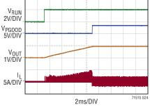
$\begin{array}{l} V_{IN} = 12 V, C_{TRACK/SS} = 0.1 \mu F \\ R_{OUT} = 60 \Omega, \ L = 0.15 \mu H, \ f_{SW} = 1 M Hz \\ R_{FB1} = 10 k \Omega, \ R_{FB2} = 10 k \Omega \\ C_{OUT} = 100 \mu F + 2 \times 330 \mu F \end{array}$
