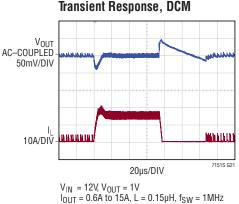
$\begin{array}{l} V_{IN} = 12 V, V_{OUT} = 1 V \\ I_{OUT} = 0.6A \ to \ 15A, \ L = 0.15 \mu H, \ f_{SW} = 1 M H z \\ R_{ITH} = 22.1 k \Omega, \ C_{ITH} = 220 p F, \ C_{ITHP} = 22 p F \\ R_{FB1} = 10 k \Omega, \ R_{FB2} = 10 k \Omega \\ C_{OUT} = 100 \mu F + 2 \times 330 \mu F \end{array}$
