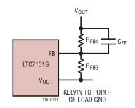
Figure 1. Setting the Output Voltage Differentially
