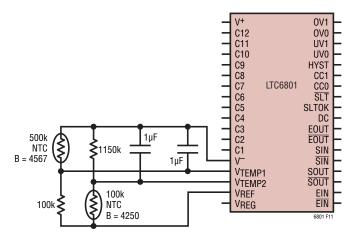
Figure 11. Sensing Both Upper and Lower Temperature Thresholds. This Example Monitors a -20°C to +60°C Window Detector. The Thermistors Should Be in Close Proximity
