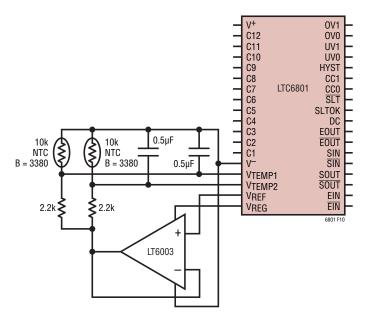
Figure 10. Buffering V<sub>REF</sub> for Higher-Current Sensors. Two Independent Probes With a +70°C Trip Point
