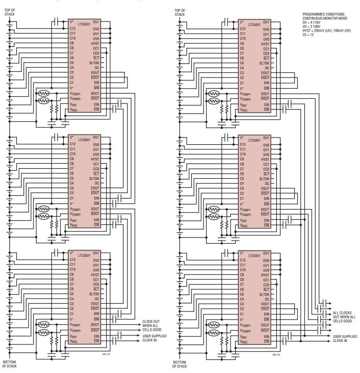
Figure 2. Serial Connection of Status Lines for Multiple LTC6801s on the Same PCB (Simplified Schematic, Not All Components Shown)
