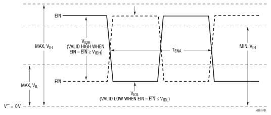
Figure 1. Differential Input Specifications
