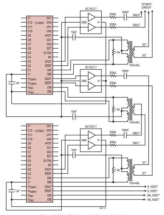
Figure 12. Using Transformers for Galvanic Isolation
