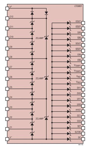
Figure 6. Internal Protection Structures
