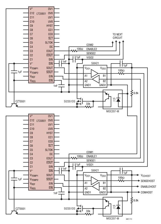
Figure 13. IC to IC Communication Using Data Isolators
