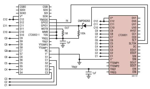
Figure 7. Interconnection of an LTC6802-1 and LTC6801 for Self Test.
