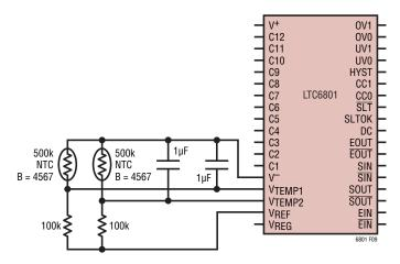
Figure 9. Driving Thermistors Directly from V<sub>REF</sub>. Two Independent Probes With a +60°C Trip Point
