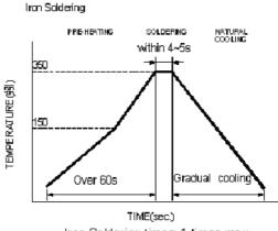
Iron Soldering times: 1 times max.
