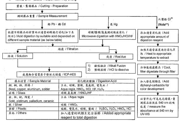
Note\*\*: (1) 針對非金屬材料加入鹼性消化液,加熱至 90~95℃ 萃取. / For non-metallic material, add alkaline digestion reagent and
