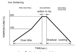
Iron Soldering times: 1 times max.
