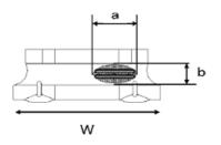
Exposed wire tolerance limit of coating resin part on product side.
