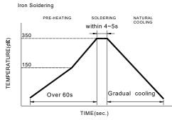
Iron Soldering times: 1 times max.
