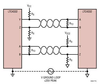
Figure 15. Resistor Bias Network
