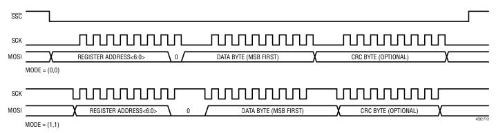
Figure 13. Control Interface Write Transfer
