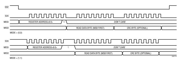
Figure 14. Control Interface Read Transfer
