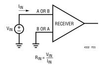
Figure 3. Receiver Input Current and Input Resistance
