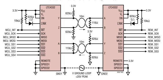
BYPASS CAPACITORS OMITTED FOR CLARITY
