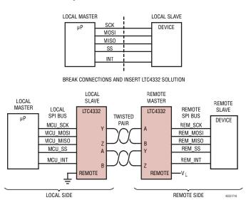
Figure 10. LTC4332 Solution Inserted Into a SPI Network
