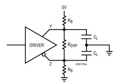
Figure 4. Driver Loading for  $I_{CC}$  Measurements
