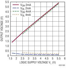
SCK, MISO, and  $\overline{INT}$  Inputs  $V_{IL}$  and  $V_{IH}$  vs  $V_L$  Supply
