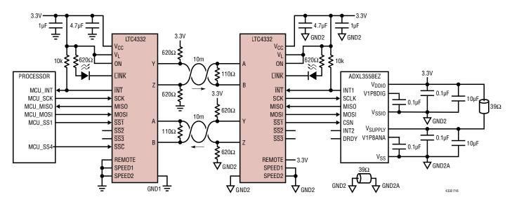
Figure 16. Extending an ADXL355BEZ Accelerometer for Remote Sensing
