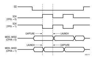
Figure 11. SPI Mode Waveform
