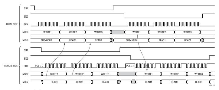
Figure 12.  $\overline{SS1}$  and  $\overline{SS2}$  Transfer. (REM\_SS1\_POL, REM\_SS1\_PHA) = (0,0). (REM\_SS2\_POL, REM\_SS2\_PHA) = (1,1). WORD\_LENGTH = 8
