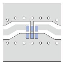
Line width to be designed to match  $50\Omega$  characteristic impedance, depending on PCB material and thickness.
