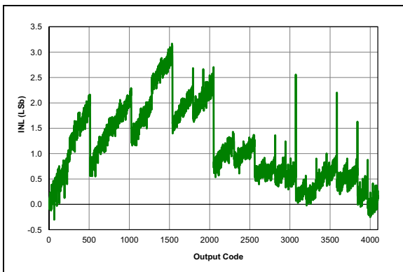
FIGURE 32-95: ADC 12-bit Mode, Single-Ended INL, V_{DD} = 5.5V , T_{AD} = 1\ \mu S , 25^\circ C .
