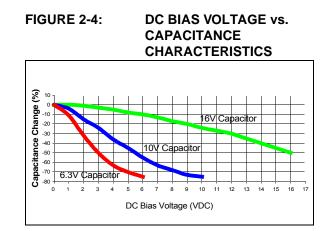
When selecting a ceramic capacitor to be used with the internal voltage regulator, it is suggested to select a high-voltage rating, so that the operating voltage is a small percentage of the maximum rated capacitor voltage. For example, choose a ceramic capacitor rated at 16V for the 2.5V or 1.8V core voltage. Suggested capacitors are shown in Table 2-1.
