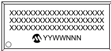
28-Lead SOIC (7.50 mm)
