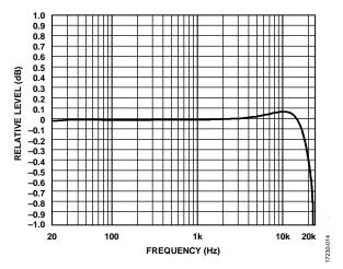
Figure 13. Relative Level vs. Frequency at -10 dBFS Normalized,  $32 \times$  Decimation,  $f_S = 48$  kHz
