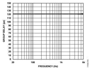
Figure 17. Group Delay vs. Frequency,  $f_S = 48$  kHz,  $16 \times$  Decimation
