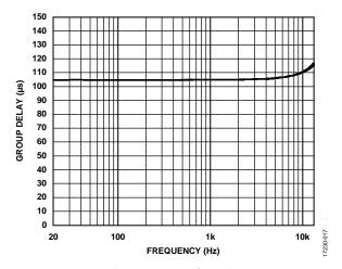
Figure 16. Group Delay vs. Frequency,  $f_s = 48$  kHz,  $32 \times$  Decimation
