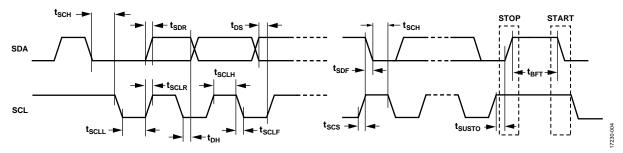
Figure 3. I<sup>2</sup>C Slave Port Timing Specifications
