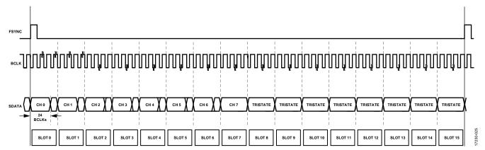
Figure 24. TDM-16, Default Channel Assignments, Left Justified Zero BCLK Delay, Normal Clock Polarity
