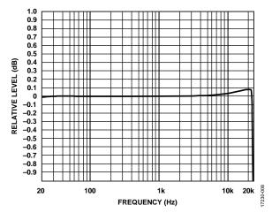
Figure 7. Relative Level vs. Frequency at -10 dBFS Normalized, 64× Decimation,  $f_S = 48$  kHz
