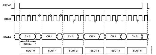
Figure 22. TDM-6, Hardware Mode, SCL = 0, SDA = x,  $f^{C}$  Mode, One BCLK Delay, Normal Clock Polarity, Default Channel Assignments
