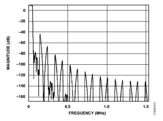
Figure 12. Magnitude vs. Frequency, 48 kHz Output, 32× Decimation
