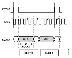
Figure 25. TDM-2, I<sup>2</sup>C Mode, One BCLK Delay, Normal Clock Polarity, Default Channel Assignments
