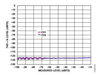
Figure 11. THD + N Level vs. Measured Level, 1 kHz, Unweighted, 64× Decimation, Fifth Order,  $f_S = 48$  kHz
