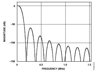
Figure 14. Magnitude vs. Frequency, 48 kHz Output, 16× Decimation
