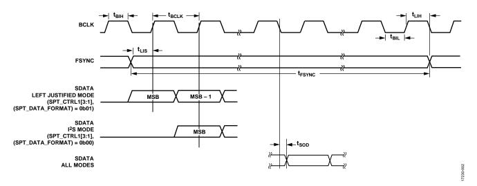
Figure 2. Serial Port Timing Specifications
