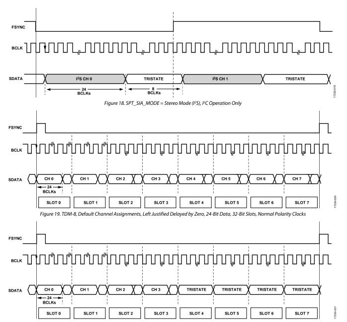
Figure 20. TDM-8, Left Justified Zero BCLK Delay, Only Channel 0 to Channel 3 Enabled
