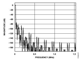
Figure 10. Magnitude vs. Frequency, 48 kHz Output, 64× Decimation
