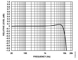
Figure 15. Relative Level vs. Frequency at -10 dBFS Normalized,  $16 \times$  Decimation,  $f_S = 48$  kHz
