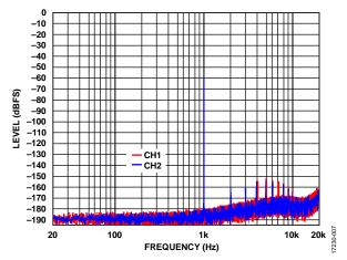
Figure 6. FFT,  $f_S = 48 \text{ kHz}$ , -60 dBFS Input,  $64 \times \text{Decimation}$ , Fifth Order
