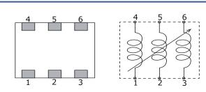
The pin numbers shown here are for reference purposes only. Confirm the actual pin number arrangement with the exchanged specification documents.
