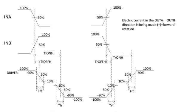
Fig.1 switching characteristics waveform
