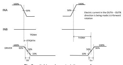
Fig.2 switching characteristics waveform
