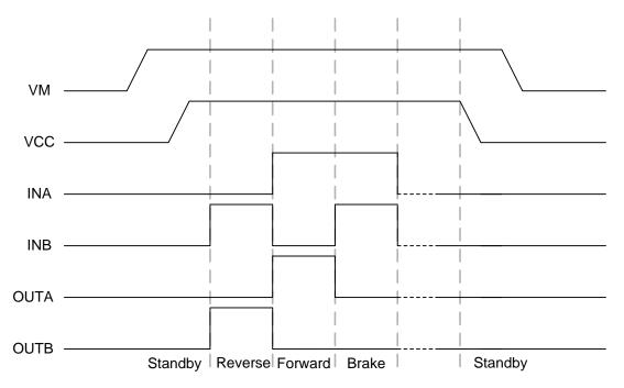
Note: VM & VCC power on have no timing sequence VM & VCC power off have no timing sequence
