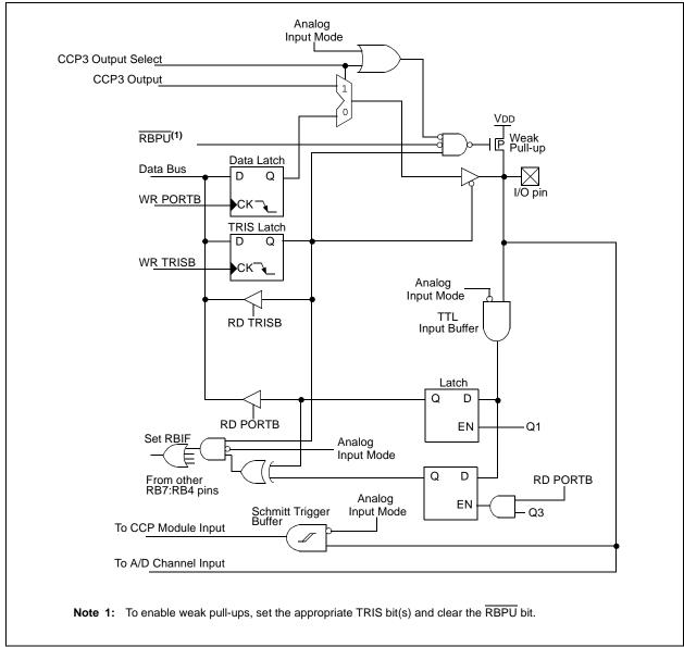
FIGURE 5-14: BLOCK DIAGRAM OF RB6/PGC PIN
