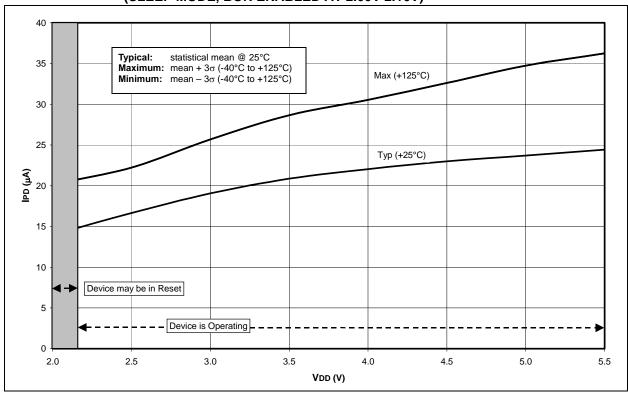
FIGURE 19-18: IPD A/D, -40°C TO +125°C (SLEEP MODE, A/D ENABLED – NOT CONVERTING)
