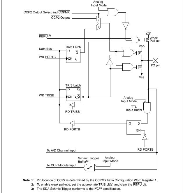
FIGURE 5-12: BLOCK DIAGRAM OF RB4/AN11 PIN
