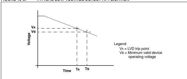
FIGURE 15-3: TYPICAL LOW-VOLTAGE DETECT APPLICATION
