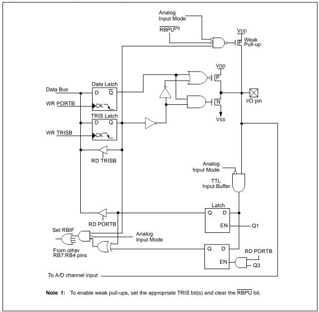
FIGURE 5-13: BLOCK DIAGRAM OF RB5/AN13/CCP3 PIN
