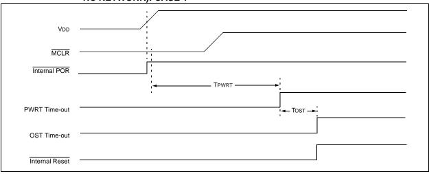
FIGURE 15-9: TIME-OUT SEQUENCE ON POWER-UP (MCLR TIED TO VDD THROUGH RC NETWORK): CASE 2
