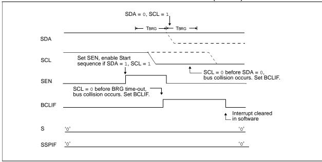
FIGURE 10-28: BRG RESET DUE TO SDA ARBITRATION DURING START CONDITION
