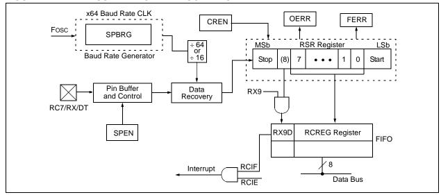
FIGURE 11-5: ASYNCHRONOUS RECEPTION
