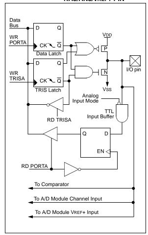
FIGURE 5-3: **BLOCK DIAGRAM OF RA2/AN2/VREF-/CVREF PIN** Data Bus Q D V<sub>DD</sub> WR **PORTA** CK 飞Q̄ Data Latch D Q RA2/AN2/VREF-/ WR TRISA CVREF pin CK~ Q TRIS Latch VSS Analog Input Mode TTL Input Buffer **RD TRISA** Q D EN < **RD PORTA** To Comparator To A/D Module VREF-To A/D Module Channel Input **CVROE CVREF**
