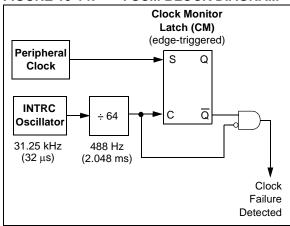
The FSCM function is enabled by setting the FCMEN bit in Configuration Word Register 2.
