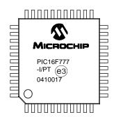
44-Lead QFN (8x8x0.9 mm)
