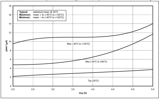
FIGURE 19-16:  $\triangle$ IPD LVD vs. VDD (SLEEP MODE, LVD = 2.00V-2.12V)
