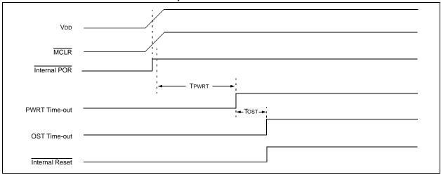
FIGURE 15-8: TIME-OUT SEQUENCE ON POWER-UP (MCLR TIED TO VDD THROUGH RC NETWORK): CASE 1
