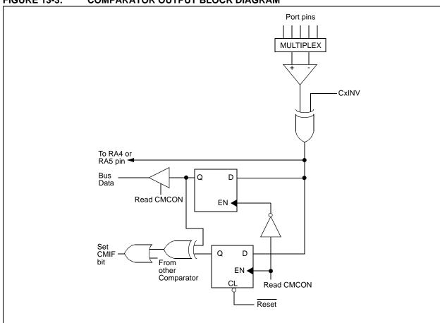
FIGURE 13-3: COMPARATOR OUTPUT BLOCK DIAGRAM
