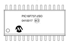
28-Lead SSOP (5.30 mm)
