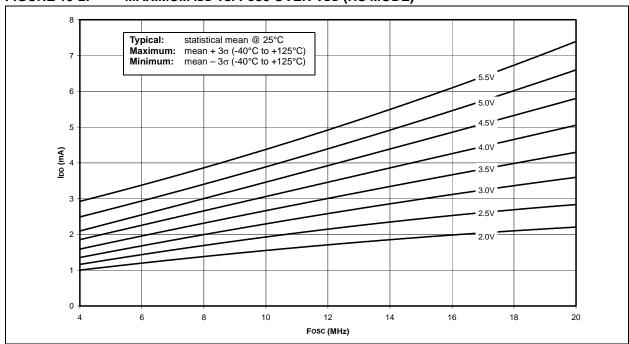
FIGURE 19-3: TYPICAL IDD vs. FOSC OVER VDD (XT MODE)
