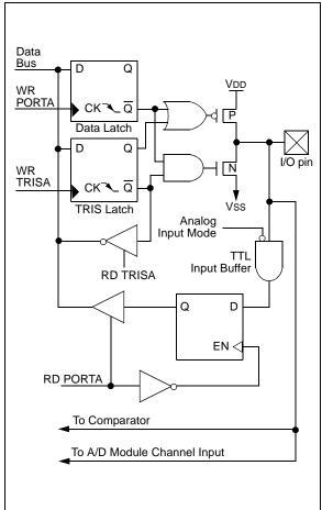
FIGURE 5-2: BLOCK DIAGRAM OF RA3/AN3/VREF+ PIN
