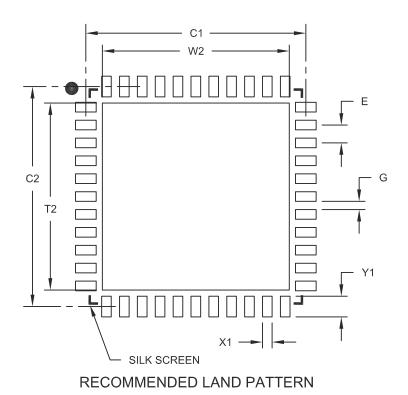
Units MILLIMETERS **Dimension Limits** MIN NOM MAX Contact Pitch Ε 0.65 BSC Optional Center Pad Width 6.80 W2 Optional Center Pad Length T2 6.80 C1 8.00 Contact Pad Spacing Contact Pad Spacing C2 8.00 0.35 Contact Pad Width (X44) X1
