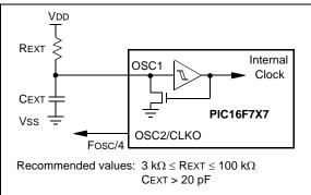
The RCIO Oscillator mode (Figure 4-5) functions like the RC mode, except that the OSC2 pin becomes an additional general purpose I/O pin. The I/O pin becomes bit 6 of PORTA (RA6).
