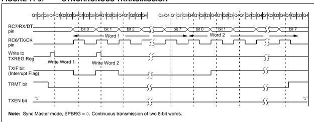
FIGURE 11-10: SYNCHRONOUS TRANSMISSION (THROUGH TXEN)
