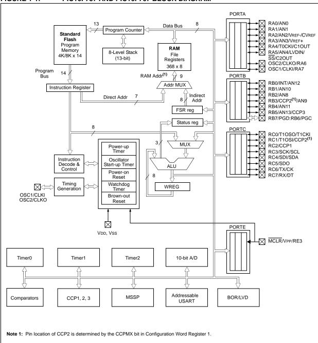
FIGURE 1-1: PIC16F737 AND PIC16F767 BLOCK DIAGRAM
