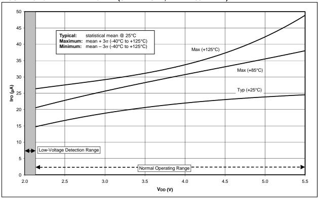
FIGURE 19-17:  $\triangle$ IPD BOR vs. VDD, -40°C TO +125°C (SLEEP MODE, BOR ENABLED AT 2.00V-2.16V)
