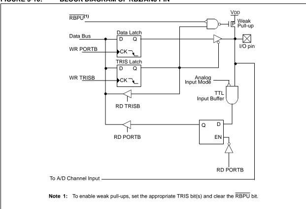
FIGURE 5-11: BLOCK DIAGRAM OF RB3/CCP2<sup>(1)</sup>/AN9 PIN
