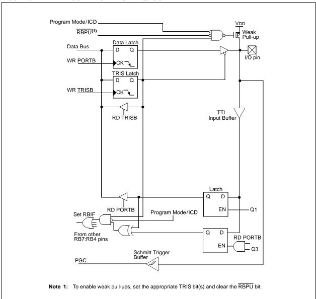
**FIGURE 5-15: BLOCK DIAGRAM OF RB7/PGD PIN** Port/Program Mode/ICD\_ PGD \_\_\_\_\_ RBPU<sup>(1)</sup> Data Latch Data Bus D WR PORTB CK \ TRIS Latch WR TRISB TTL Input Buffer **RD TRISB** PGD DRVEN Latch D **RD PORTB** ΕN Program Mode/ICD Set RBIF D From other RB7:RB4 pins **RD PORTB** ΕN Q3 PGD<del></del>◀
