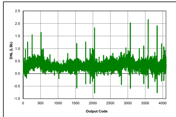
FIGURE 31-94: ADC 12-bit Mode, Single-Ended DNL, V_{DD} = 5.5V , T_{AD} = 4\ \mu S , 25^\circ C .
