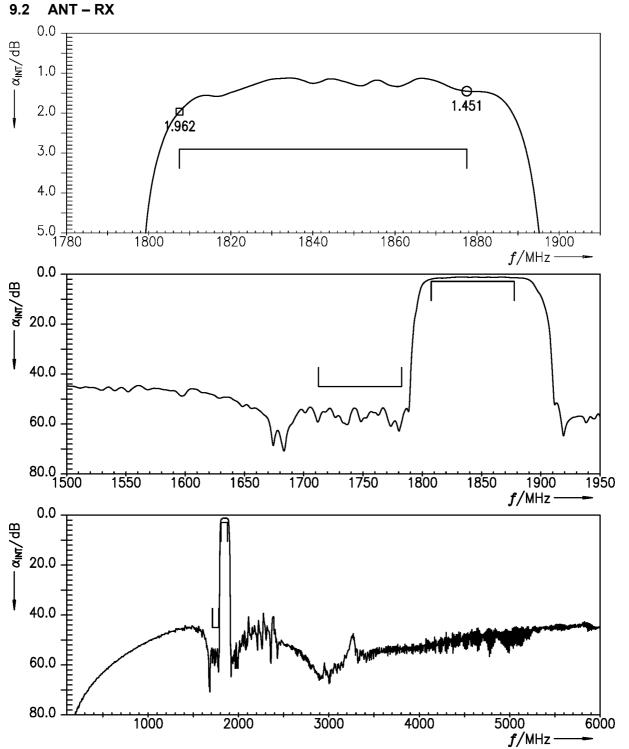
**Figure 7:** Attenuation (LTE) (integration window = 5 MHz) ANT – RX.
