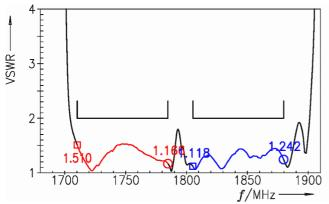
Figure 10: Reflection coefficient at ANT port.
