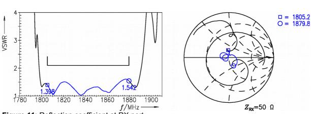
Figure 11: Reflection coefficient at RX port.
