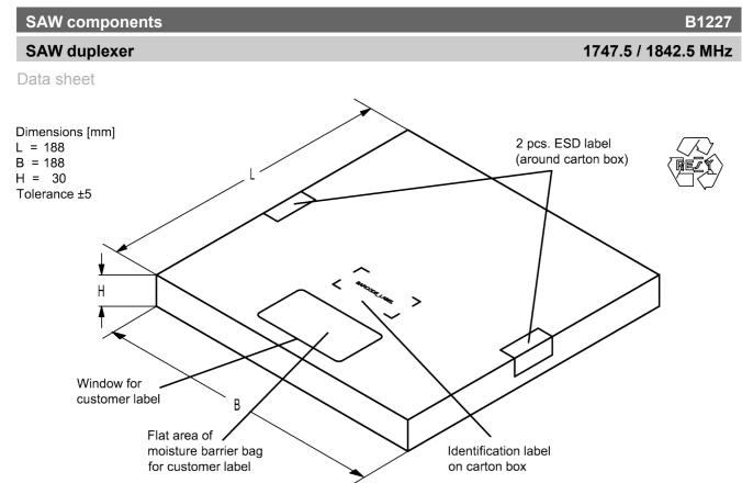
Figure 17: Drawing of folding box for reel with diameter of 180 mm.
