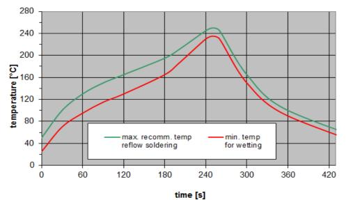
**Figure 21:** Recommended reflow profile for convection and infrared soldering – lead-free solder.
