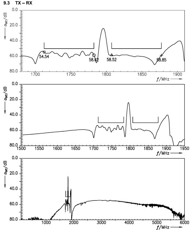
Figure 8: Isolation (LTE) (integration window = 5 MHz) TX – RX.
