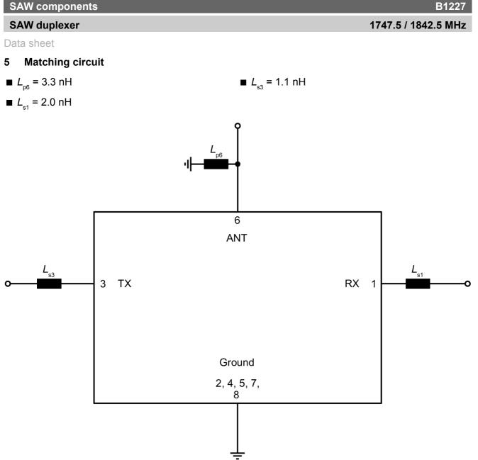
Figure 3: Schematic of matching circuit.
