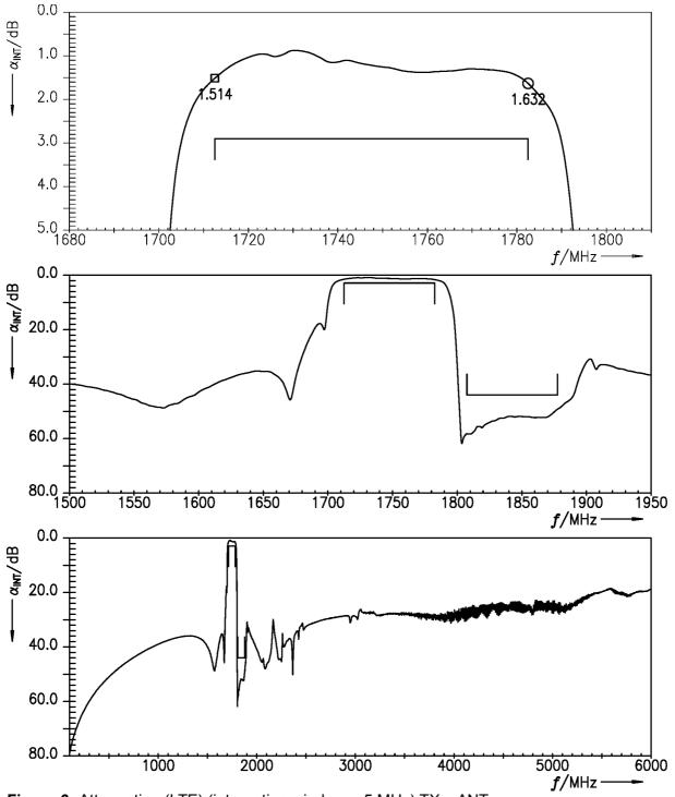
Figure 6: Attenuation (LTE) (integration window = 5 MHz) TX – ANT.
