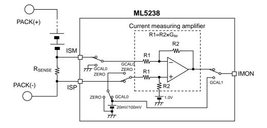
The circuit of current measuring amplifier is shown below.
