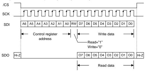
Set the RW bit "0" to write data, and set the RW bit "1" to read data.
