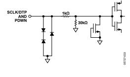
Figure 10. Equivalent SCLK/DTP and PDWN Input Circuit
