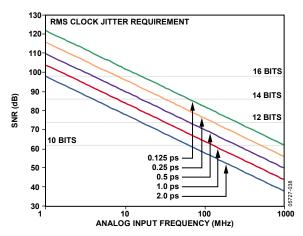
Figure 57. Ideal SNR vs. Input Frequency and Jitter
