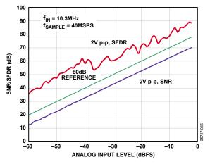
Figure 27. SNR/SFDR vs. Analog Input Level,  $f_{IN} = 10.3$  MHz,  $f_{SAMPLE} = 40$  MSPS
