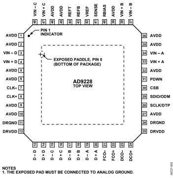
Figure 5. 48-Lead LFCSP Pin Configuration, Top View
