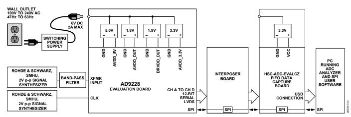
Figure 71. Evaluation Board Connection
