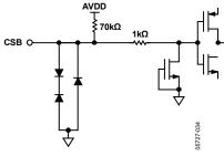
Figure 12. Equivalent CSB Input Circuit
