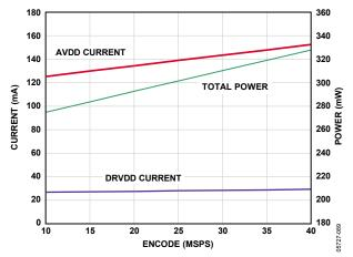
Figure 58. Supply Current vs.  $f_{SAMPLE}$  for  $f_{IN} = 10.3$  MHz,  $f_{SAMPLE} = 40$  MSPS
