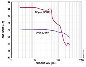
Figure 35. SNR/SFDR vs. Frequency,  $f_{SAMPLE} = 65 \text{ MSPS}$
