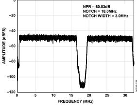
Figure 41. Noise Power Ratio (NPR), f<sub>SAMPLE</sub> = 65 MSPS
