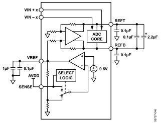
Figure 65. External Reference Operation
