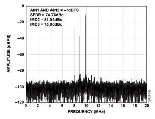
Figure 32. Two-Tone 32k FFT with  $f_{\rm IN1}$  = 70 MHz and  $f_{\rm IN2}$  = 71 MHz,  $f_{\rm SAMPLE}$  = 40 MSPS
