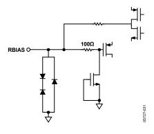
Figure 11. Equivalent RBIAS Circuit
