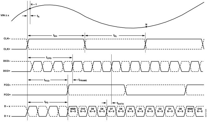
Figure 2. 12-Bit Data Serial Stream, MSB First (Default)
