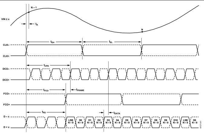
Figure 4. 12-Bit Data Serial Stream, LSB First
