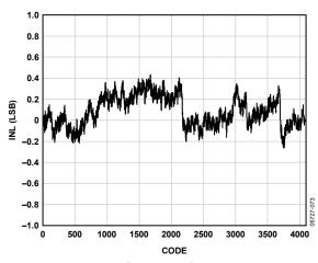
Figure 37. INL,  $f_{IN} = 2.4$  MHz,  $f_{SAMPLE} = 65$  MSPS
