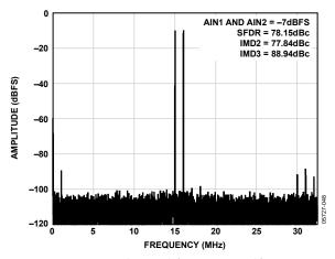
Figure 33. Two-Tone 32k FFT with  $f_{\rm IN1}=15$  MHz and  $f_{\rm IN2}=16$  MHz,  $f_{\rm SAMPLE}=65$  MSPS
