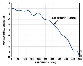
Figure 42. Full-Power Bandwidth vs. Frequency, f<sub>SAMPLE</sub> = 65 MSPS
