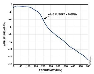
Figure 72. Evaluation Board Full-Power Bandwidth
