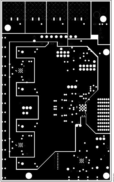
Figure 80. Evaluation Board Layout, Power Plane
