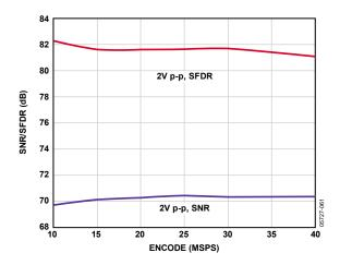
Figure 24. SNR/SFDR vs. Encode,  $f_{IN} = 35$  MHz,  $f_{SAMPLE} = 40$  MSPS
