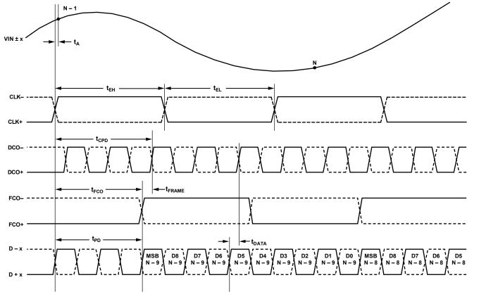
Figure 3. 10-Bit Data Serial Stream, MSB First
