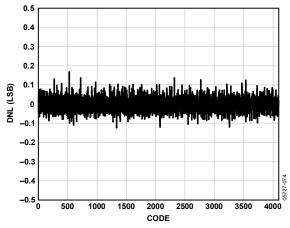
Figure 38. DNL,  $f_{IN} = 2.4 \text{ MHz}$ ,  $f_{SAMPLE} = 65 \text{ MSPS}$
