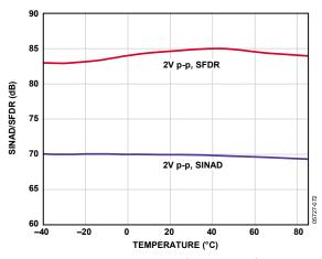
Figure 36. SINAD/SFDR vs. Temperature,  $f_{IN} = 10.3$  MHz,  $f_{SAMPLE} = 65$  MSPS
