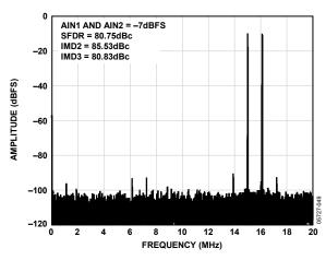
Figure 31. Two-Tone 32k FFT with  $f_{\rm IN1}$  = 15 MHz and  $f_{\rm IN2}$  = 16 MHz,  $f_{\rm SAMPLE}$  = 40 MSPS
