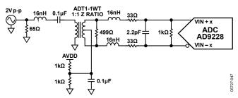
Figure 49. Differential Transformer-Coupled Configuration for IF Applications
