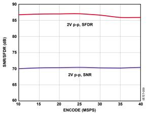
Figure 23. SNR/SFDR vs. Encode,  $f_{IN} = 10.3 \text{ MHz}$ ,  $f_{SAMPLE} = 40 \text{ MSPS}$
