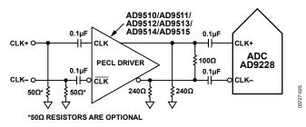
Figure 53. Differential PECL Sample Clock
