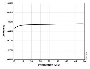
Figure 39. CMRR vs. Frequency,  $f_{SAMPLE} = 65 \text{ MSPS}$
