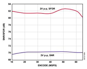
Figure 26. SNR/SFDR vs. Encode,  $f_{IN} = 35$  MHz,  $f_{SAMPLE} = 65$  MSPS
