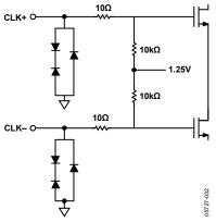
Figure 7. Equivalent Clock Input Circuit
