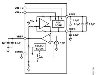
Figure 64. Internal Reference Configuration
