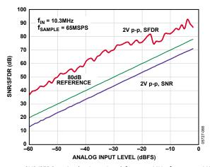
Figure 29. SNR/SFDR vs. Analog Input Level,  $f_{\text{IN}} = 10.3 \text{ MHz}$ ,  $f_{\text{SAMPLE}} = 65 \text{ MSPS}$
