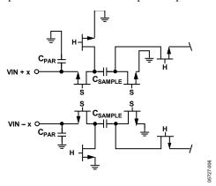
Figure 43. Switched-Capacitor Input Circuit
