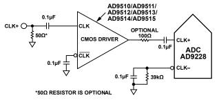
Figure 55. Single-Ended 1.8 V CMOS Sample Clock
