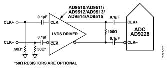
Figure 54. Differential LVDS Sample Clock
