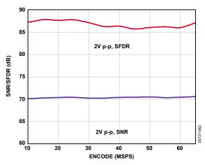
Figure 25. SNR/SFDR vs. Encode,  $f_{IN} = 10.3 \text{ MHz}$ ,  $f_{SAMPLE} = 65 \text{ MSPS}$
