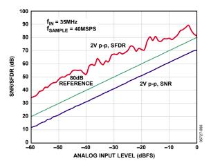
Figure 28. SNR/SFDR vs. Analog Input Level,  $f_{IN} = 35$  MHz,  $f_{SAMPLE} = 40$  MSPS
