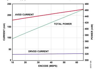
Figure 59. Supply Current vs.  $f_{SAMPLE}$  for  $f_{IN} = 10.3$  MHz,  $f_{SAMPLE} = 65$  MSPS
