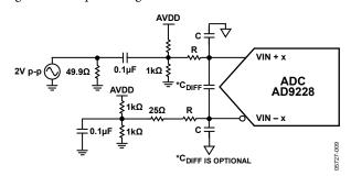
Figure 50. Single-Ended Input Configuration
