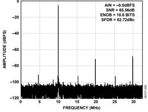
Figure 22. Single-Tone 32k FFT with  $f_{\text{IN}}$  = 250 MHz,  $f_{\text{SAMPLE}}$  = 65 MSPS
