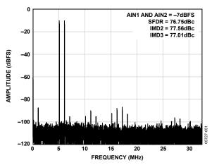
Figure 34. Two-Tone 32k FFT with  $f_{\rm IN1}=70$  MHz and  $f_{\rm IN2}=71$  MHz,  $f_{\rm SAMPLE}=65$  MSPS
