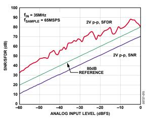
Figure 30. SNR/SFDR vs. Analog Input Level,  $f_{IN} = 35$  MHz,  $f_{SAMPLE} = 65$  MSPS
