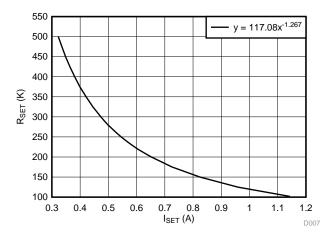
Figure 7. Linear Regulator Current Limit Vs Resistor
