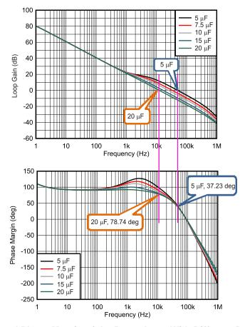
Figure 13. Gain and Phase Margin of the Boost Loop With Different Boost Capacitance ( $V_{IN}$  = 12 V,  $V_{OUT}$  =18.2 V,  $I_{LOAD}$  = 1 A,  $f_{SW}$  = 1 MHz, 10  $\mu$ H, Typical Bode Plot)
