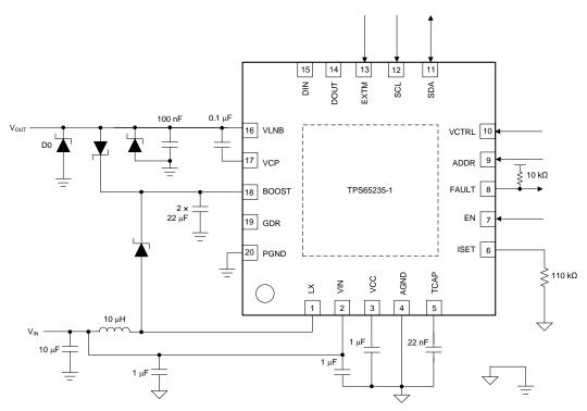
Figure 21. Application for DiSEqc1.x Support
