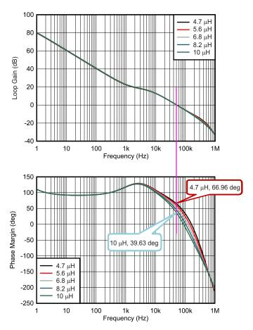
Figure 11. Gain and Phase Margin of the Boost Loop with Different Inductance  $(V_{IN} = 12 \text{ V}, V_{OUT} = 18.2 \text{ V}, I_{LOAD} = 1 \text{ A}, f_{SW} = 1 \text{ MHz}, 5 \mu\text{F}, Typical Bode Plot})$
