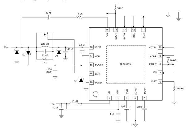
Figure 38. Application Schematic for DiSEqc2.x Support
