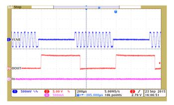
Figure 39. DOUT Tone Detection Output
