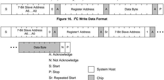
Figure 17. I<sup>2</sup>C Read Data Format
