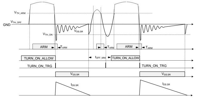
Figure 6. SR Turn-On Algorithm
