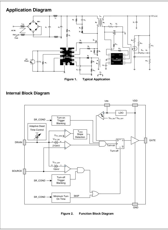
FAN6240 — Secondary-Side Synchronous Rectifier Controller for Flyback Converters
