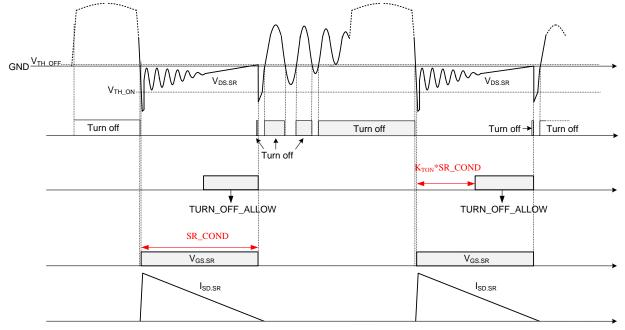
Figure 7. SR Turn-Off Algorithm
