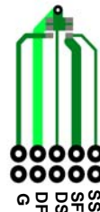
b. 175\text{ }^\circ\text{C}/\text{W} when mounted on a minimum pad of 2 oz copper
