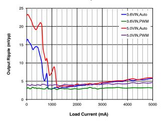
Figure 7. Output Ripple vs. Load Current
