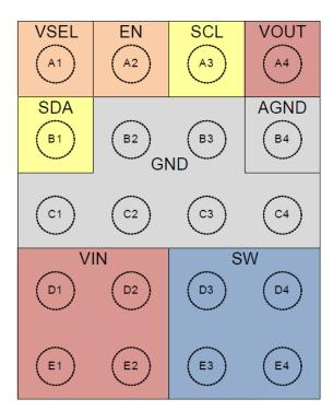
Figure 2. Pin Assignment (Top View)
