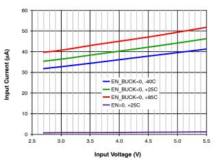
Figure 10. Shutdown Current vs. Input Voltage, Over–Temperature
