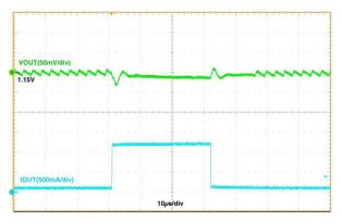
Figure 11. Load Transient,  $I_{OUT}$  = 0.1 A  $\Leftrightarrow$  1.2 A, Auto PFM Mode,  $T_R$  =  $T_F$  = 100 ns
