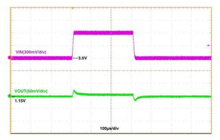
Figure 12. Line Transient, V<sub>IN</sub> = 3.0 V  $\Leftrightarrow$  3.6 V, T<sub>R</sub> = T<sub>F</sub> = 10 µs, I<sub>OUT</sub> = 500 mA
