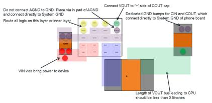
Figure 24. Remote Sensing Guidance, Top Layer
