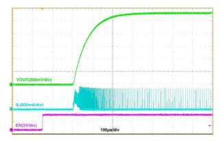
Figure 13. Startup,  $R_{load}$  = 50  $\Omega$
