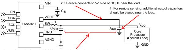
3. The trace resistance between FAN53200 and CPU should not exceed 30 m  $\!\Omega\!.$
