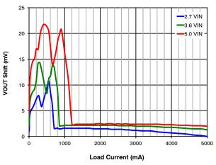
Figure 4. Output Regulation vs. Load Current and Input Voltage
