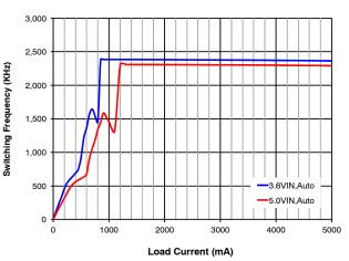
Figure 8. Frequency vs. Load Current
