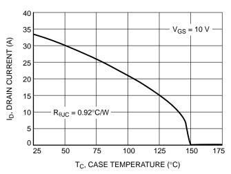
Figure 5. Maximum Continuous  $I_D$  vs. Case Temperature
