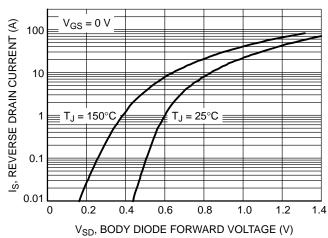
Figure 7. Forward Diode
