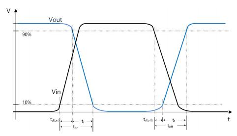
Figure 3. Timing Measurement Variable Definition
