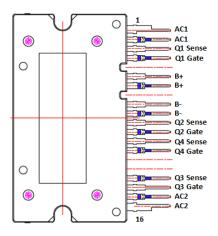
Figure 1. Pin Configuration
