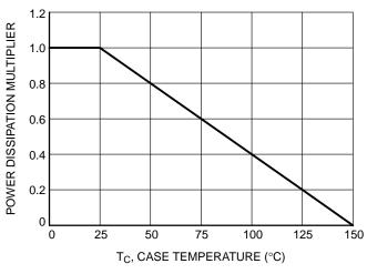
Figure 4. Normalized Power Dissipation vs. Case
