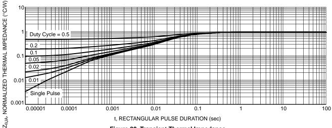
Figure 20. Transient Thermal Impedance
