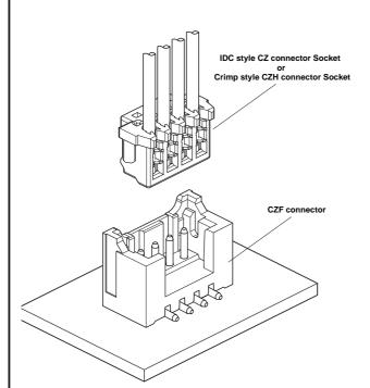
The SMT top entry type headers that can be mated with the 1.5 mm pitch CZ connector socket are on the lineup.
