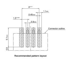
Note: 1. The above figure is the figure viewed from the connector mounting side.
