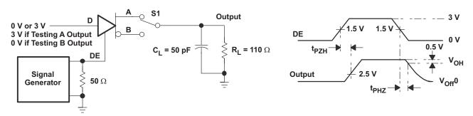
Figure 12. Driver Enable and Disable Test Circuit and Waveforms, High Output
