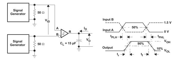
Figure 16. Receiver Switching Test Circuit and Waveforms
