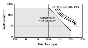
Figure 24. Cable Length vs Data Rate Characteristic
