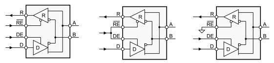
Figure 22. Half-Duplex Transceiver Configurations
