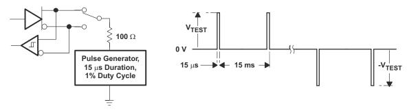
Figure 20. Test Circuit and Waveforms, Transient Overvoltage Test
