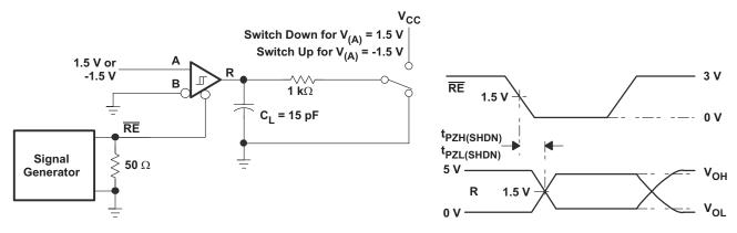
Figure 19. Receiver Enable From Shutdown Test Circuit and Waveforms
