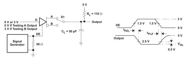
Figure 13. Driver Enable and Disable Test Circuit and Waveforms, Low Output
