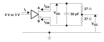
Figure 8. Driver Test Circuit, V<sub>OD</sub> and V<sub>OC</sub> Without Common-Mode Loading
