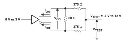
Figure 9. Driver Test Circuit,  $V_{\text{OD}}$  With Common-Mode Loading
