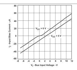
Figure 1. Bus Input Current versus Bus Input Voltage
