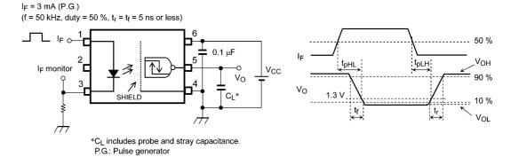
Fig. 13.1.7 Switching Time Test Circuit and Waveform
