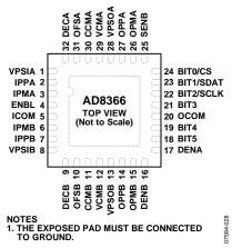
Figure 4. Pin Configuration
