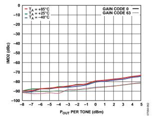
Figure 27. IMD2 vs. Output Power (P<sub>OUT</sub>) at Minimum and Maximum Gain Codes, 10 MHz Frequency
