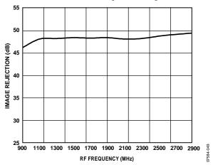
Figure 53. Image Rejection vs. RF Frequency
