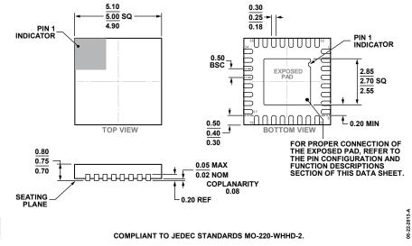
Figure 63. 32-Lead Lead Frame Chip Scale Package [LFCSP] 5 mm × 5 mm Body and 0.75 mm Package Height (CP-32-21) Dimensions shown in millimeters
