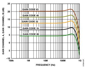
Figure 6. Frequency Response vs. Gain Code
