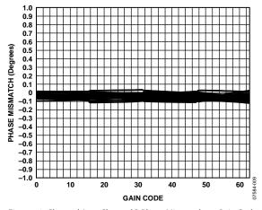
Figure 10. Channel A-to-Channel B Phase Mismatch vs. Gain Code, 2 V p-p Output
