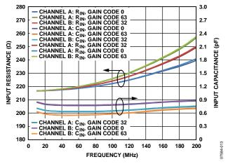
Figure 31. Differential Parallel Input Resistance and Capacitance vs. Frequency
