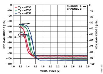
Figure 22. HD3/HD2 vs. V<sub>OCM</sub> at 10 MHz, Gain Code 0, 2 V p-p Output
