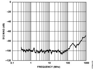
Figure 43. Reverse Isolation (S12) vs. Frequency
