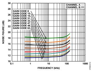
Figure 33. Noise Figure vs. Frequency
