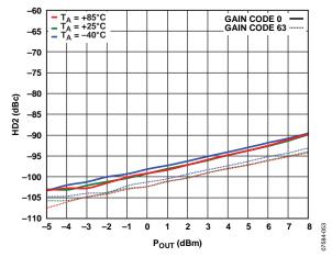
Figure 25. HD2 vs. Output Power ( $P_{\text{OUT}}$ ) at Gain Code 0 and Gain Code 63, 10 MHz Frequency
