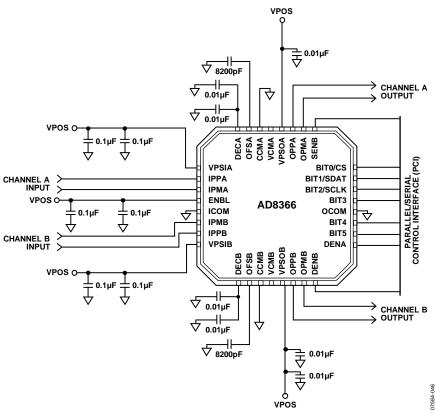
Figure 50. Basic Connections
