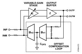
Figure 47. Differential Offset Correction Loop
