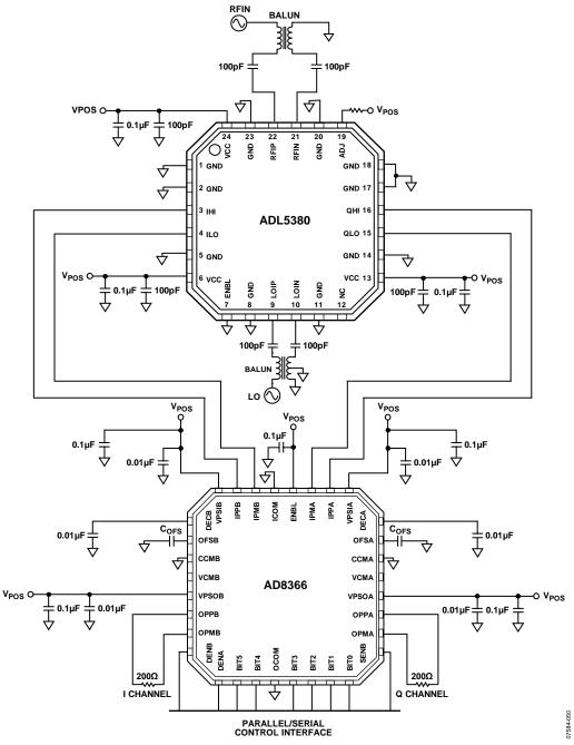
Figure 56. ADL5380 and AD8366 Interface Block Diagram
