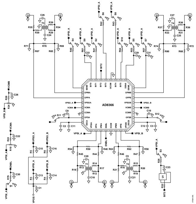
Figure 60. Evaluation Board Schematic
