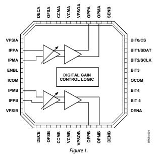
The output common-mode voltage defaults to  $V_{POS}/2$  but can be programmed via the VCMA and VCMB pins over a range of voltages. The input common-mode voltage also defaults to  $V_{POS}/2$  but can be driven down to 1.5 V. A built-in, dc offset compensation loop can be used to eliminate dc offsets from prior stages in the signal chain. This loop can also be disabled if dc-coupled operation is desired.
