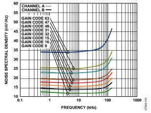
Figure 32. Noise Spectral Density vs. Frequency
