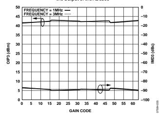
Figure 55. OIP3 on Low Frequency, 2 V p-p Composite
