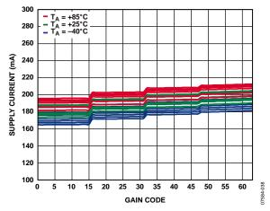
Figure 29. Supply Current vs. Gain Code at 10 MHz
