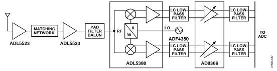
Figure 51. Direct Conversion Receiver Block Diagram
