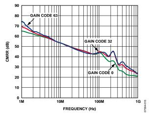
Figure 39. Common-Mode Rejection Ratio (CMRR) vs. Frequency
