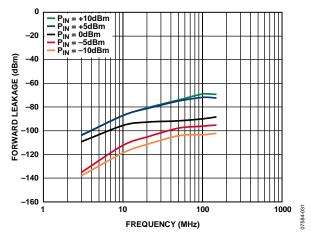
Figure 40. Forward Leakage vs. Frequency, Part Disabled
