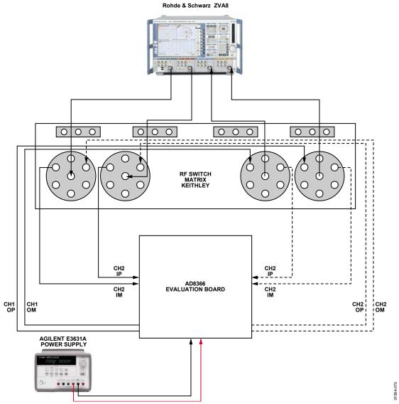
Figure 59. Characterization Setup, Differential Measurements
