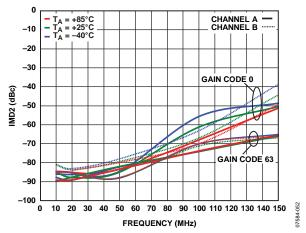
Figure 21. Two-Tone Output IMD2 vs. Frequency, Gain Code 0 and Gain Code 63, 2 V p-p Composite Output
