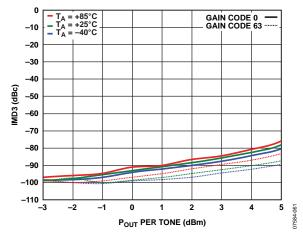
Figure 26. IMD3 vs. Output Power (P<sub>OUT</sub>) at Minimum-to-Maximum Gain Codes, 10 MHz Frequency
