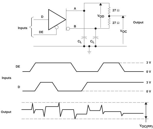
NOTES: A. Resistance values are in ohms and are 1% tolerance.
