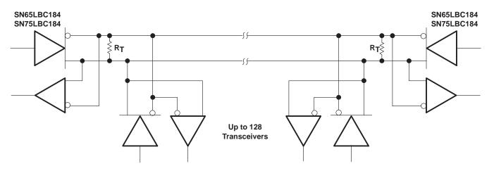
NOTE A: The line should be terminated at both ends in its characteristic impedance (R<sub>T</sub> = Z<sub>O</sub>). Stub lengths off the main line should be kept as short as possible.
