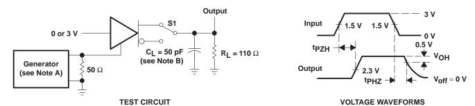
NOTES: A. The input pulse is supplied by a generator having the following characteristics: PRR = 1.25 kHz, 50% duty cycle,  $t_{\Gamma} \le 10$  ns,  $t_{f} \le 10$  ns,  $t_{O} = 50 \Omega$ .
