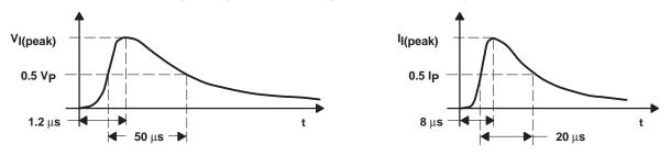
Figure 15. Short-Circuit Current Waveforms
