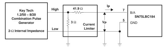
Figure 16. Overvoltage-Stress Test Circuit
