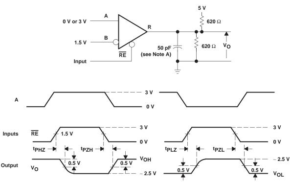
NOTE A: This value includes probe and jig capacitance ( $\pm$  10%).
