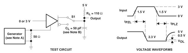
NOTES: A. The input pulse is supplied by a generator having the following characteristics: PRR = 1.25 kHz, 50% duty cycle,  $t_{\Gamma} \le 10$  ns,  $t_{f} \le 10$  ns,  $t_{O} = 50 \Omega$ .
