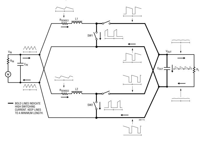
Figure 15. BOOST Converter Branch Current Waveforms
