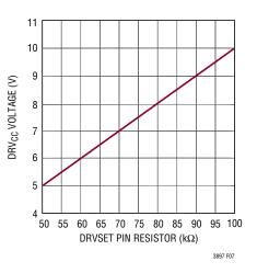
Figure 7. Relationship Between  $\text{DRV}_{\text{CC}}$  Voltage and Resistor Value at DRVSET Pin
