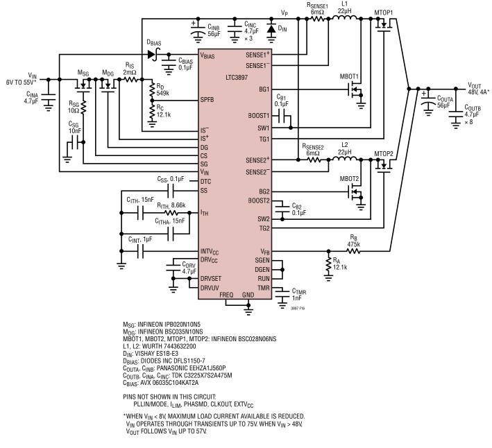
Figure 16. High Efficiency 2-Phase 48V Boost Converter with In-Rush Current Control, Overcurrent Protection, Input Voltage Surge Protection and Reverse Input Protection
