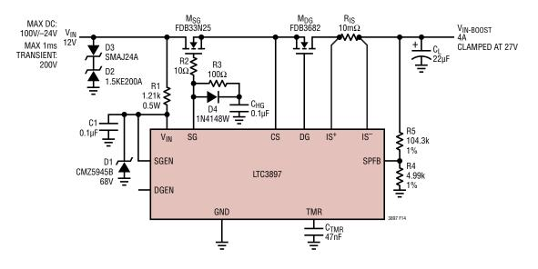
Figure 14. 4A, 12V Overvoltage and Reverse Current Protection
