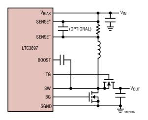
(2a) Using a Resistor to Sense Current
