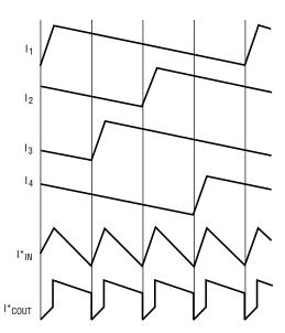
\* RIPPLE CURRENT CANCELLATION INCREASES THE RIPPLE FREQUENCY AND REDUCES THE RMS INPUT/OUTPUT RIPPLE CURRENT, THUS SAVING INPUT/OUTPUT CAPACITORS
