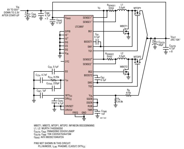
High Efficiency 2-Phase 24V Boost Converter (Input Supply Down to 2.3V After Start Up)
