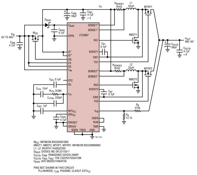
High Efficiency 2-Phase 48V Boost Converter with Reverse Input Protection (Surge Stopper Controller Not Used)
