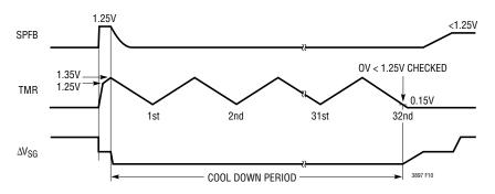
Figure 10. Auto-Retry Cool Down Timer Cycle Following Overvoltage Fault
