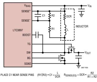
(2b) Using the Inductor DCR to Sense Current
