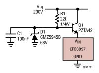
Figure 11. Buffering V<sub>IN</sub> to Extend Input Supply Range
