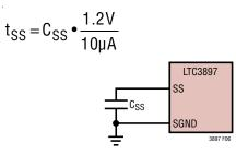
Figure 6. Using the SS Pin to Program Soft-Start
