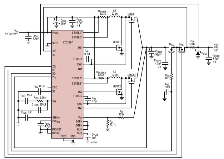
High Efficiency 2-Phase 48V Boost Converter with Overcurrent Protection (Ideal Diode and Surge Stopper Controllers at the Output)
