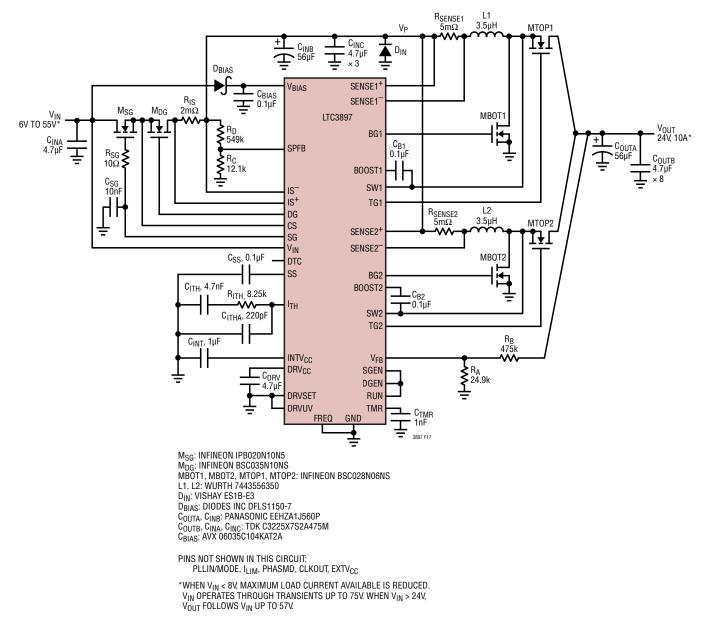
Figure 17. High Efficiency 2-Phase 24V Boost Converter with In-Rush Current Control, Overcurrent Protection, Input Voltage Surge Protection and Reverse Input Protection
