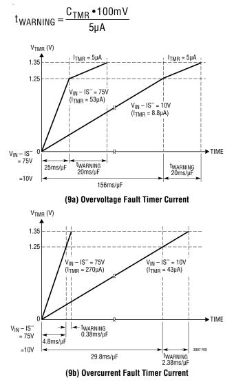
Figure 9. Fault Timer Current of the LTC3897
