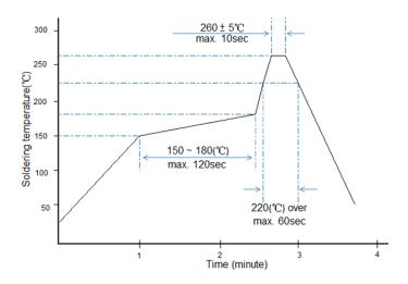
Recommended IR Reflow Soldering Profile MEET J-STD-020D
