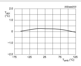
Fig 19. Typical temperature accuracy versus temperature; V<sub>CC</sub> = 3.3 V
