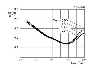
Fig 16. Shutdown mode supply current versus temperature
