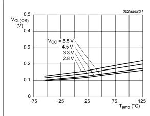
Fig 17. LOW-level output voltage on pin OS versus temperature; I<sub>OL</sub> = 4 mA
