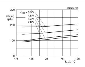
Fig 15. Average supply current versus temperature; I<sup>2</sup>C-bus active
