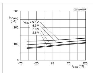
Fig 14. Average supply current versus temperature; I<sup>2</sup>C-bus inactive
