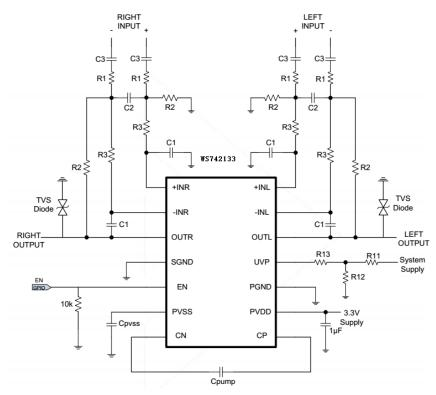
Differential-input, single-ended output, second-order filter R1=15k $\Omega$ , R2=30k $\Omega$ , R3=47k $\Omega$ , C1=33pF, C2=150pF, C3=6.8 $\mu$ F, R11=5.6k $\Omega$ , R12=2.43k $\Omega$ , R13=15K $\Omega$ , Cpvss=0.33 to 1 $\mu$ F, Cpump=0.33 to 1 $\mu$ F.
