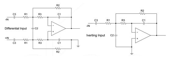
Figure 5. Second-Order Active Low-Pass Filter
