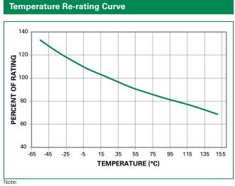
Re-rating depicted in this curve is in addition to the standard re-rating of 20% for continuous operation.
