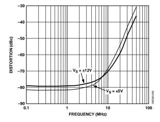
Figure 27. Third Harmonic Distortion vs. Frequency and Power Supplies,  $V_0 = 2 V p - p$
