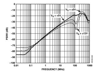
Figure 30. Positive Power Supply Rejection Ratio vs. Frequency
