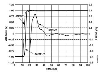
Figure 22. Settling Time (0.1%) at Various Loads
