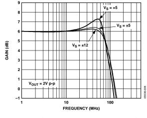
Figure 8. Large Signal Frequency Response at Various Power Supplies, G=2
