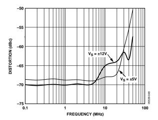
Figure 24. Second Harmonic Distortion vs. Frequency and Power Supplies,  $V_{\rm O}$  = 2 V p-p
