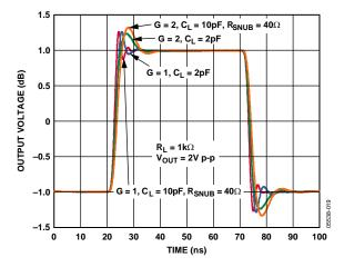
Figure 21. Large Signal Transient Response at Various Gains and 10 pF Capacitive Load Buffered by 40  $\Omega$  Resistor
