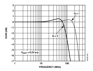
Figure 11. Small Signal Frequency Response at Various Gains
