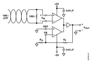
Figure 40. Differential-Mode Termination
