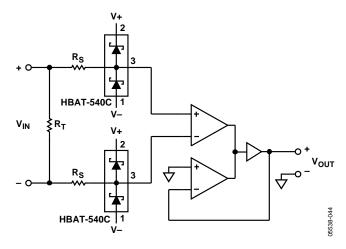
Figure 44. External Common-Mode Clamping
