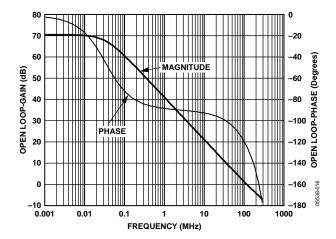
Figure 15. Open-Loop Gain and Phase Responses
