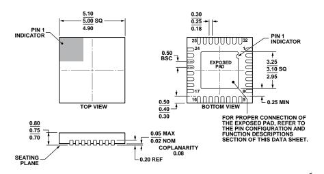
Figure 49. 32-Lead Lead Frame Chip Scale Package [LFCSP] 5 mm × 5 mm Body and 0.75 mm Package Height (CP-32-7) Dimensions shown in millimeters
