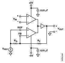
Figure 39. Basic Gain Circuit:  $V_{OUT} = V_{IN} (1 + R_F/R_G) + V_{REF}$
