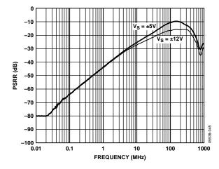
Figure 33. Negative Power Supply Rejection Ratio vs. Frequency
