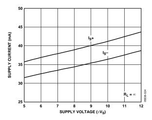
Figure 32. Power Supply Current vs. Power Supply Voltage
