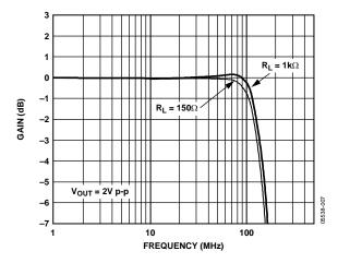
Figure 9. Large Signal Frequency Response at Various Loads
