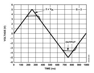
Figure 35. Output Overdrive Recovery
