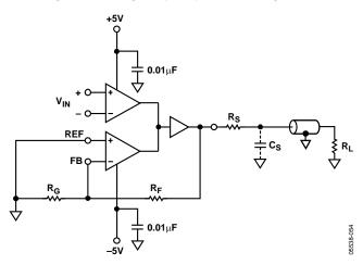
Figure 47. Driving a Doubly Terminated Cable
