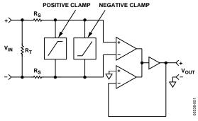
Figure 42. Differential-Mode Clamping
