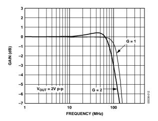
Figure 14. Large Signal Frequency Response at Various Gains
