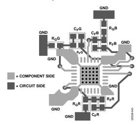
Figure 45. Recommended Layout for Feedback Loops and Grounding
