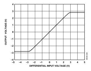
Figure 31. Differential Input Operating Range
