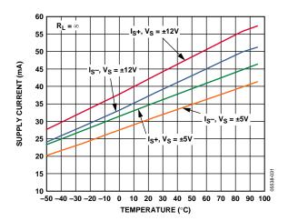
Figure 29. Power Supply Current vs. Temperature
