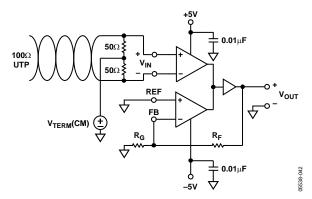
Figure 41. Common-Mode Termination
