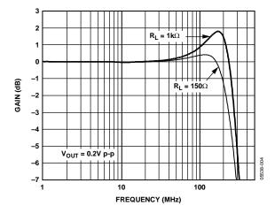
Figure 6. Small Signal Frequency Response at Various Loads
