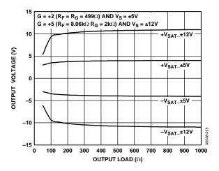
Figure 34. Output Saturation Voltage vs. Output Load
