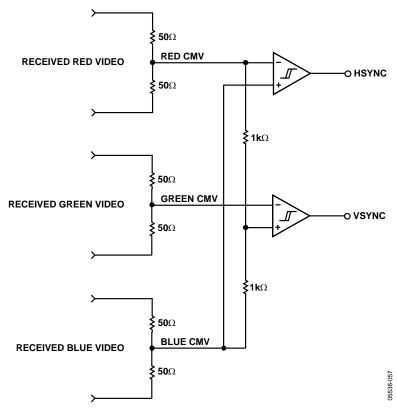
Figure 48. Extracting Sync Signals from Received Common-Mode Signals
