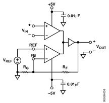
Figure 37. Basic Gain Circuit:  $V_{OUT} = (V_{IN} + V_{REF})(1 + R_F/R_G)$
