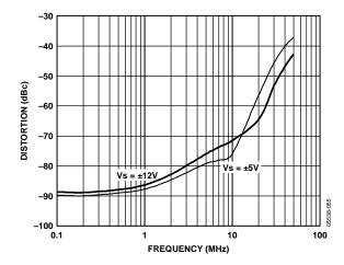
Figure 26. Third Harmonic Distortion vs. Frequency and Power Supplies,  $V_0 = 2 V p\text{-}p$ , G = 2
