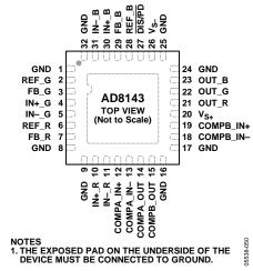
Figure 3. Pin Configuration
