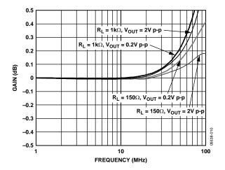
Figure 12. 0.1 dB Flatness for Various Loads and Output Amplitudes
