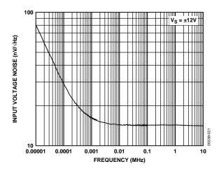
Figure 19. Input Referred Voltage Noise vs. Frequency
