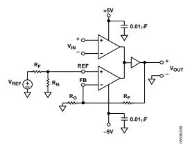
Figure 38. Basic Gain Circuit:  $V_{OUT} = V_{IN} (1 + R_F/R_G) + V_{REF}$
