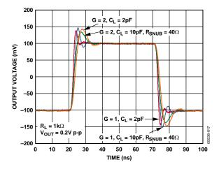
Figure 18. Small Signal Transient Response at Various Gains and 10 pF Capacitive Load Buffered by 40  $\Omega$  Resistor
