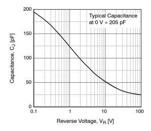
Figure 5. Typical Junction Capacitance
