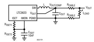
Figure 1. Output Cable Drop Compensation
