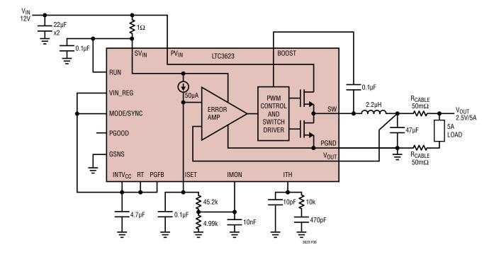
Figure 7. 12V to 3.3V 1MHz Buck Regulator with Input Supply Regulation Loop
