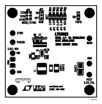
Figure 3. PCB Layout - Top Side
