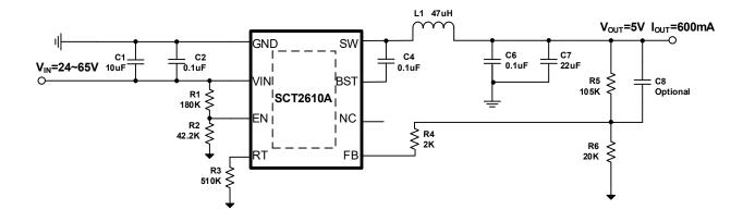
Figure 11. SCT2610A Design Example, 5V Output with Programmable UVLO
