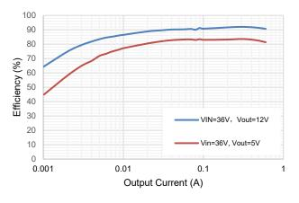
Figure 2. Efficiency vs Load Current
