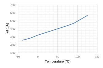
Figure 6. Shut-down Current vs Temperature
