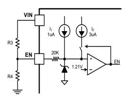
Figure 9. System UVLO by enable divide
