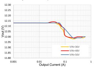
Figure 4. Load Regulation (Vout=12V)
