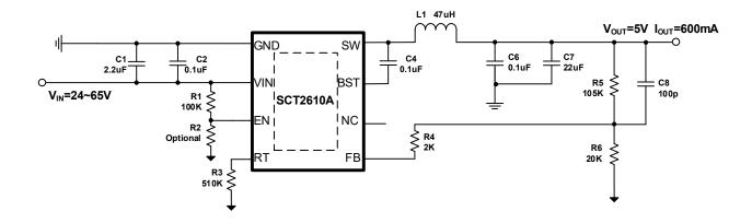
Figure 13. VOUT=5V, IOUT=0.6A Application Circuit
