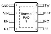
Figure 1. 8-Lead Plastic E-SOP
