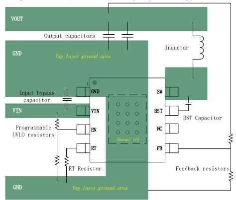
Figure 26. PCB Layout Example
