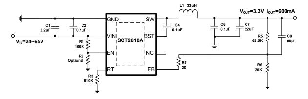
Figure 12. VOUT=3.3V, IOUT=0.6A Application Circuit
