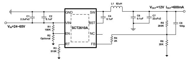
Figure 14. VOUT=12V, IOUT=0.6A Application Circuit
