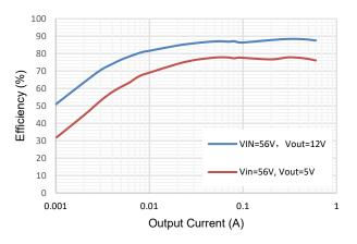
Figure 3. Efficiency vs Load Current
