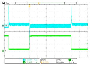
Figure 22.Load Transient (0.5A-4.5A, 250mA/us)
