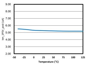
Figure 11. EN Pull-up Current vs Temperature
