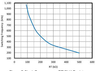
Figure 7.Clock Frequency vs RT/CLK Resistor
