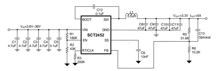
Figure 18. SCT2452 Design Example, 3.3V Output with Programmable UVLO
