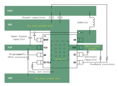
Figure 26. PCB Layout Example
