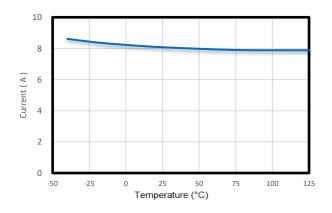
Figure 13. Peak Current Limit vs Temperature
