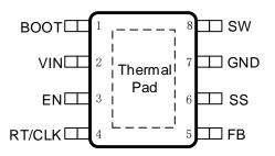
Figure 1. 8-Lead Plastic E-SOP
