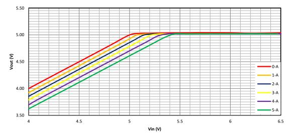
Figure 17. LDO Operation Characteristic ( Vout =5V )
