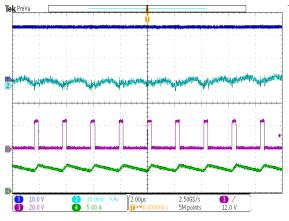
Figure 24. SW and Vout Ripple
