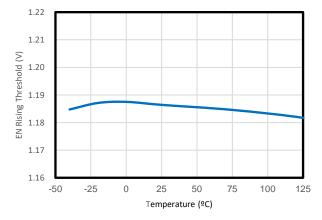
Figure 10. EN Threshold vs Temperature
