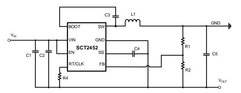
Figure 19. SCT2452 Inverting Power Supply
