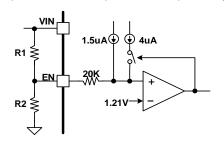
Figure 15. System UVLO by enable divide
