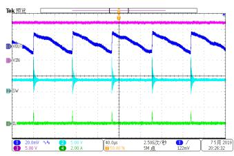
Figure 10. SW node Waveform and Output Ripple VIN=12V, IOUT=10mA
