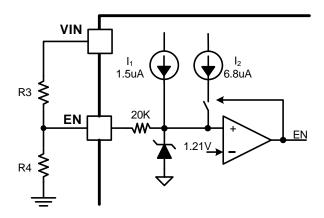
Figure 7. Adjustable VIN UVLO
