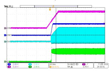
Figure 11. Power Up VIN=12V, VOUT=3.3V, IOUT=3A
