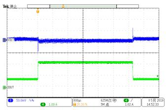
Figure 14. Load Transient VOUT=3.3V, IOUT=0.75A to 2.25A, SR=250mA/us
