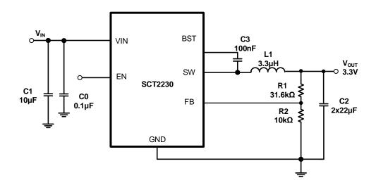
Figure 8. 12V Input, 3.3V/3A Output
