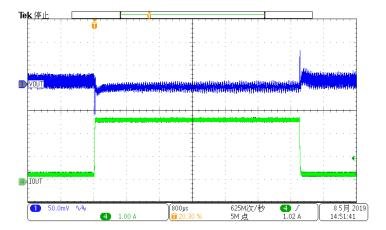
Figure 13. Load Transient VOUT=3.3V, IOUT=0.3A to 2.7A, SR=250mA/us
