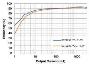
Figure 1. SCT2230 Efficiency, Vin=12V
