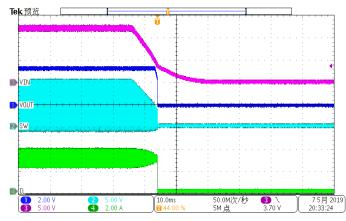
Figure 12. Power Down VIN=12V, VOUT=3.3V, IOUT=3A
