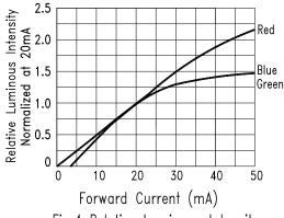
Fig.4 Relative Luminous Intensity vs. Forward Current
