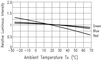
Fig.5 Luminous Intensity vs.Ambient Temperature
