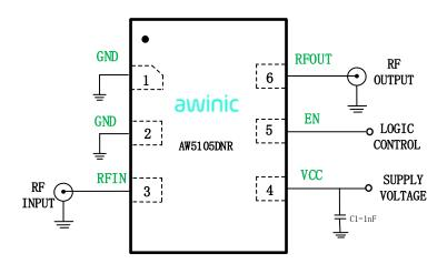
Figure 1 Typical Application Circuit of AW5105
