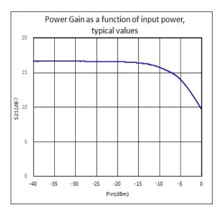
TA=25 °C, VCC=2.8 V, EN=2.8 V, Rs=Ro=50 ohm, for typical values (unless otherwise noted).
