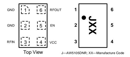
Figure 2 Pin Configuration and Top Mark
