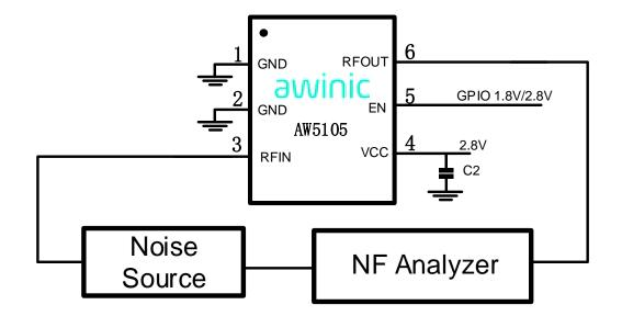
**Figure7 Circuit for Noise Figure test**
