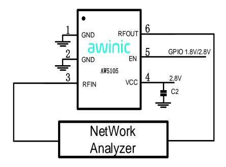
Figure 6 Circuit for S Parameter test
