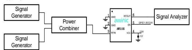
Figure8 Circuit for intermodulation distortion test
