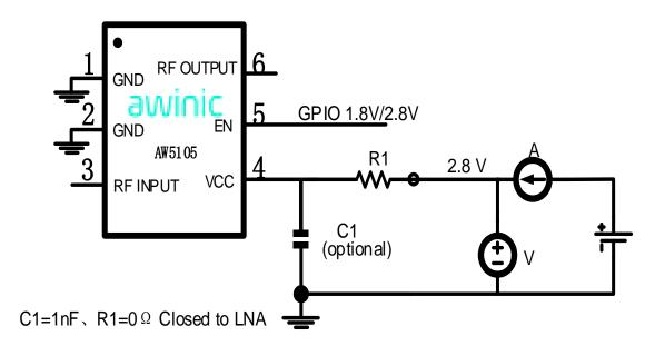
Figure5 Circuit for DC test
