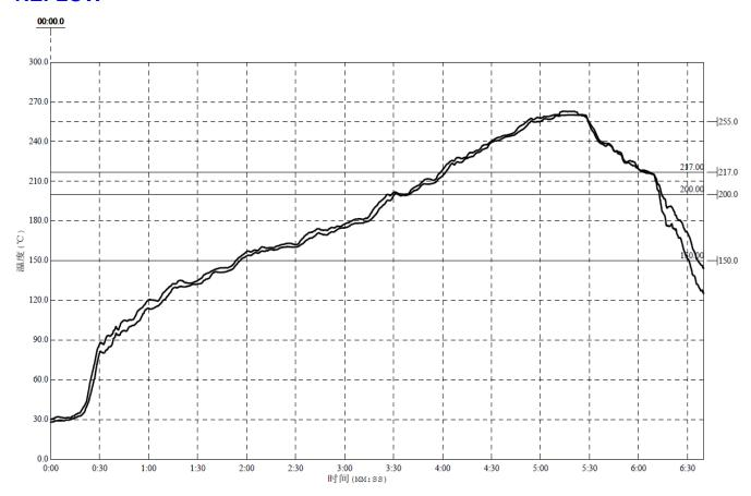
Figure 13 Package Reflow Oven Thermal Profile
