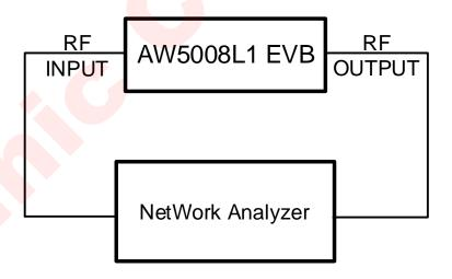
Figure 6 AW5008L1 S-parameter Measurement Diagram
