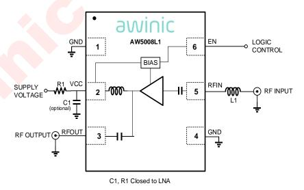
Figure 1 Typical Application Circuit of AW5008L1
