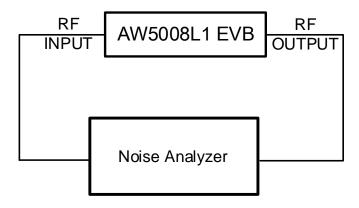
Figure 7 AW5008L1 Noise Figure Measurement Diagram
