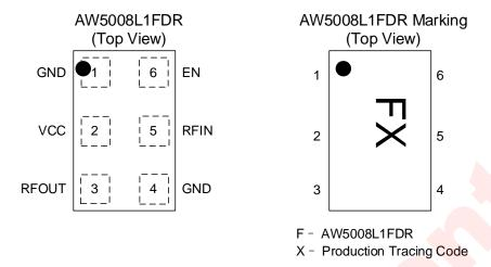
Figure 2 Pin Configuration and Top Mark
