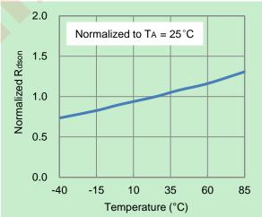
Figure 8 Normalized R<sub>dson</sub> vs. Temp. (I<sub>OUT</sub> = 1A)
