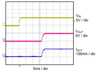
Figure 14 Power-up ( $C_{OUT} = 1\mu F$ , 100mA load)
