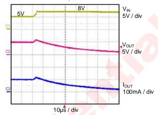
**Figure 15** Power-up ( $C_{OUT} = 100 \mu F$ , 100mA load)
