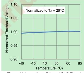
Figure 12 Normalized External OVP Threshold
