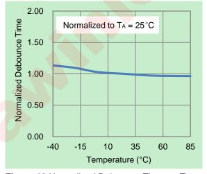
Figure 13 Normalized Debounce Time vs. Temp.
