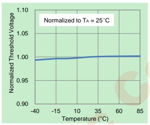
Figure 11 Normalized Internal OVP Threshold
