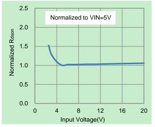
Figure 9 Normalized  $R_{dson}$  vs. Input Voltage ( $I_{OUT} = 1A$ )
