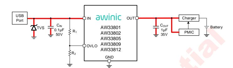
Figure 5 AW338XX typical application circuit(using external OVP threshold)
