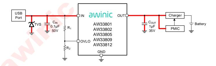
Figure 1 AW338XX typical application circuit
