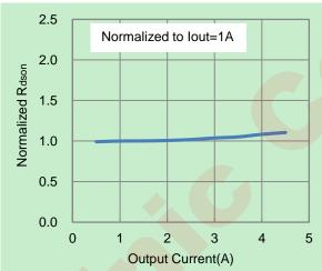
Figure 7 Normalized Rdson vs. Output Current
