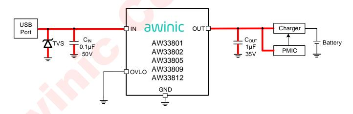
Figure 4 AW338XX typical application circuit(using default OVP threshold)
