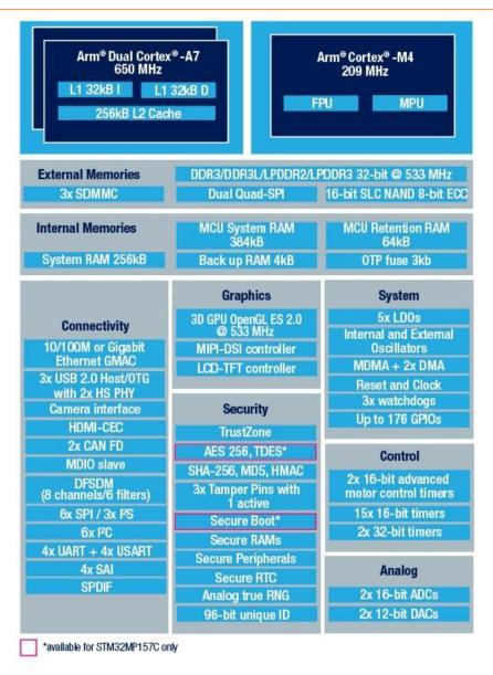
Figure 1-5 STM32MP157 Block Diagram
