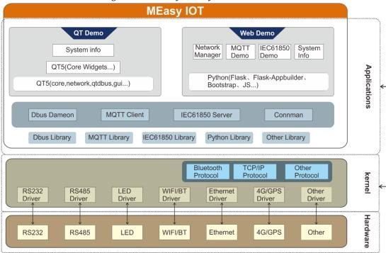
Figure 1-13 MEasy-IOT System Structure
