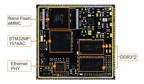
Figure 1-6 MYC-YA157C CPU Module
