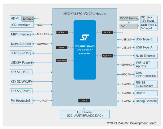
Figure 1-9 MYD-YA157C Development Board Function Block Diagram
